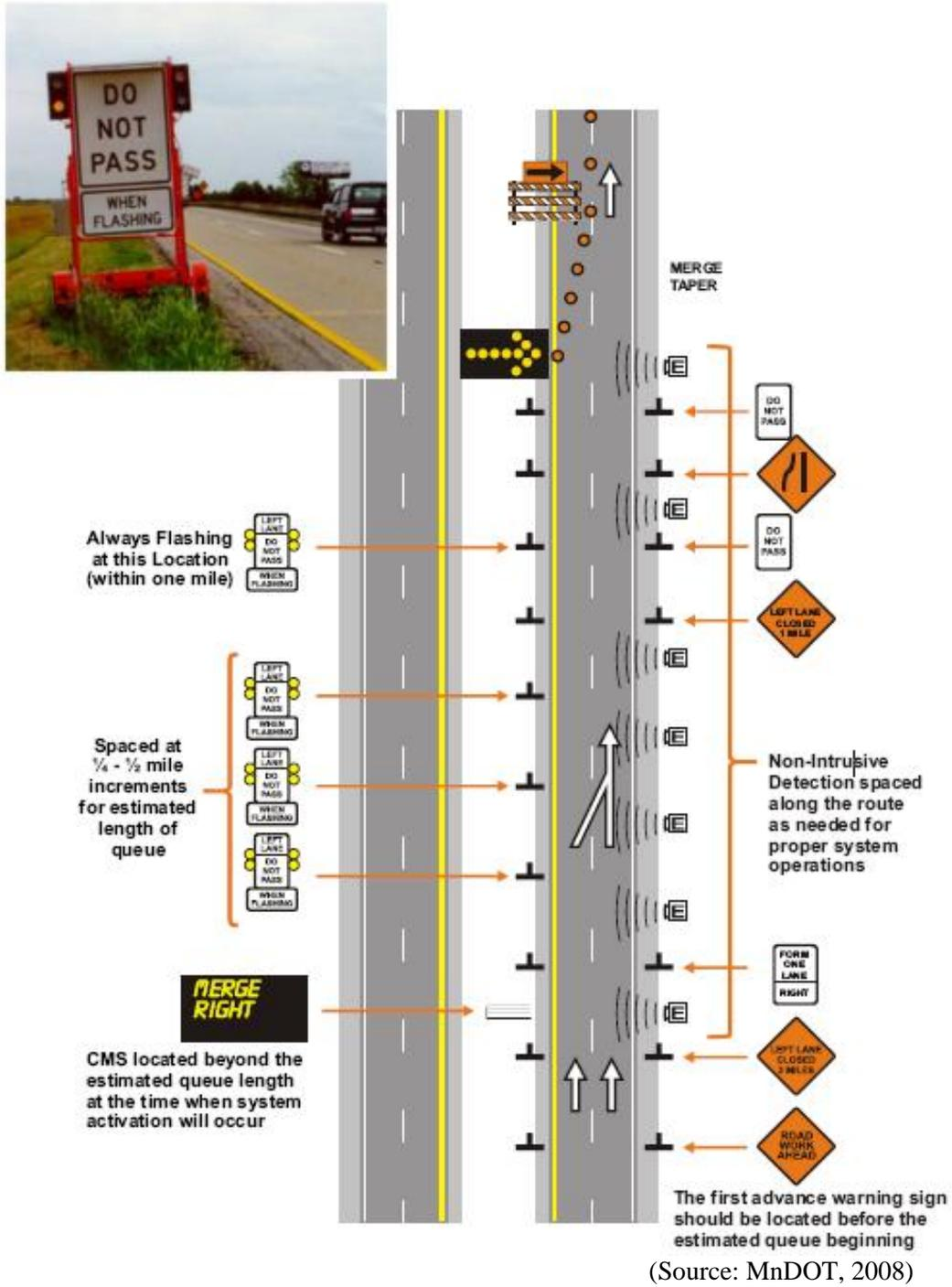
Figure 2 Layout of an Early Merge System
